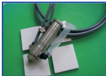
Figure 1: Preparation of samples for antimicrobial efficiency testing.
