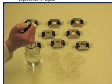
Figure 2: Preparation of samples for efficiency testing regarding degradation of algae.
